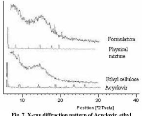
Fig. 7. X-ray diffraction pattern of Acyclovir, ethyl cellulose (EC), physical mixture and formulation
